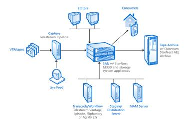
The combination of Telestream workflow and transcode products and StorNext SAN file system creates a powerful platform for enhancing workflow efficiency and performance. The example diagram above depicts a common broadcast workflow environment.
